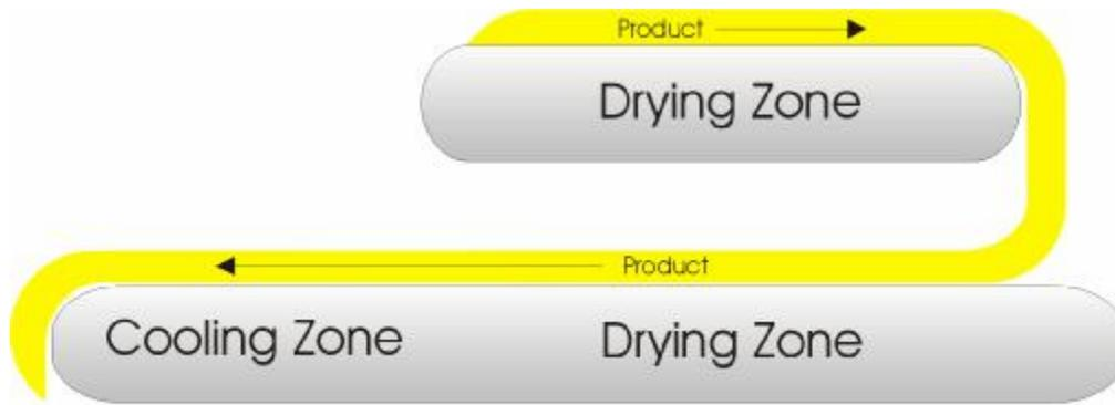
Figure1: Illustration of a combination horizontal dryer/cooler.
