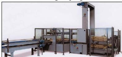
allows layer transfer during product accumulation, effectively staging and stacking layers every 15 seconds (four layers per minute). Products are repositioned to any required orientation during high-speed operation with the servo-operated overhead orienter.
