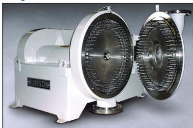
A new 24-inch (610 mm) sanitary stainless steel centrifugal impact mill Model CIM-24-SS from Munson Machinery provides coarse to fine grinding (325 mesh) of friable materials into controlled particle sizes, as well
