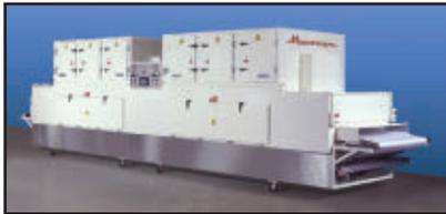
Macrowave dryers, according to Radio Frequency, eliminate surface checking and control moisture and color.
